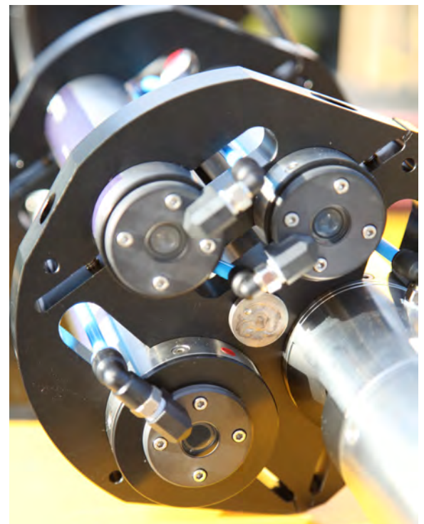
One of the 3 possible flexible sensor mountings
