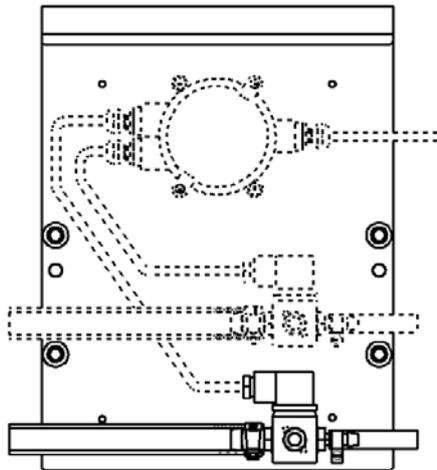
Mounting plate with two solenoid valves and a M12 multiplexer.
