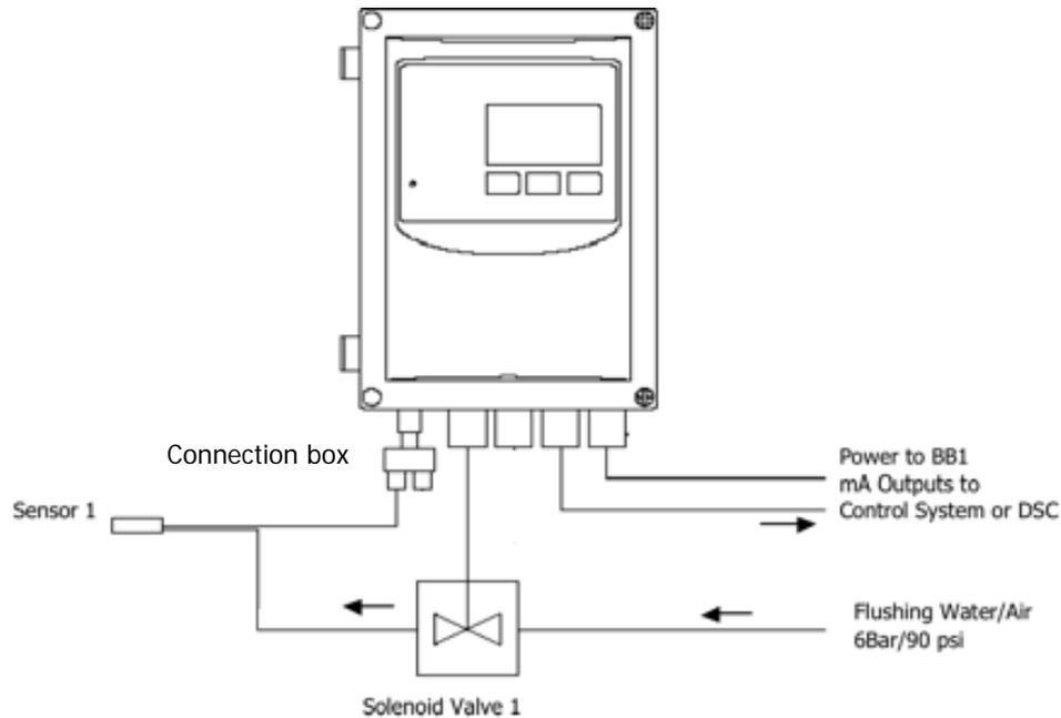
**Figure 1** Connection of BB1 Control box with one sensor and two flushing valves
