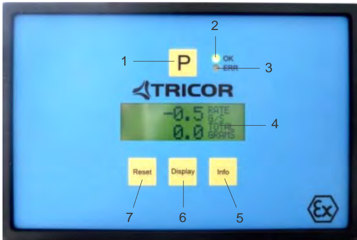
Fig. 2: Operating Elements of TCE 8***-L*-Ex
