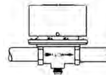
With Body Tapped for Direct Installation (Series FS1, FS5 and FS6) FS6
